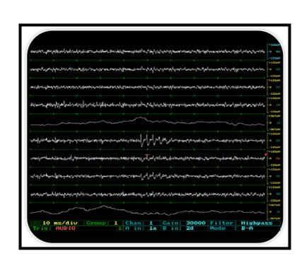
A typical display from the digital oscilloscope showing simultaneous single unit recording on 8 channels (1-4 and 6-9), and EEG recording on 2 channels (5 and 10). The electrode configuration was tetrode, and channels 1-4 are the signals from tetrode 1, with channels 6-9 the signals from tetrode 2.
